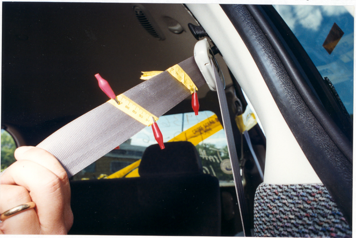
101. Close-up of an abrasion on the upper portion of restraint webbing near the D-ring.
